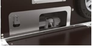
**O Electric winch, 12v with remote control** Electric winch, mounted as shown is powered by a fully fitted 12v battery pack. Full remote control is via a wander lead. Winch features free line spool and roller guides. Mains charger supplied.
